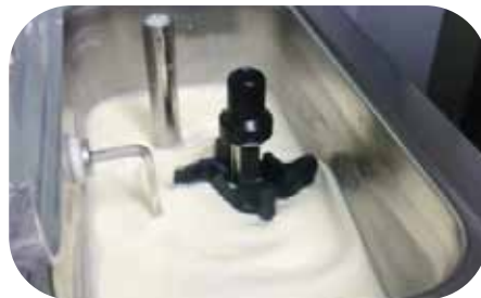
Agitator Mix low & out sensors
